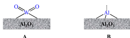
Scheme 2. Probable Structures of (A) Isolated \text{WO}_4 or (B) Tetrahedral \text{AlO}_4 Species on \text{Pd}-\text{WO}_x/\text{Al}_2\text{O}_3
